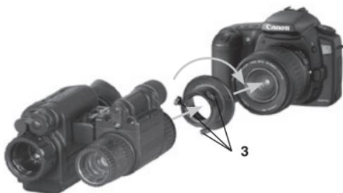
**Figure 2-8. Mounting Camera to the ATN FIITS-14**
