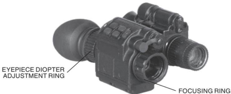
**Figure 3-4. Focus Adjustment of TVU**
