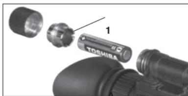
**Figure 2-2. AA Battery Installation**
