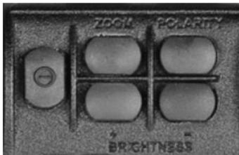
**Figure 3-3. Switchboard of Thermal Vision Unit**
