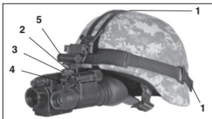
**Figure 2-5. Attaching FIITS-14 to Helmet Mount**
