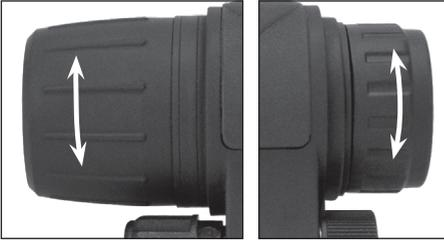
To focus the Viper X-1, first you will need to adjust the diopter. Simply turn the diopter clockwise until it stops. Then, while looking through the diopter at an object, slowly turn the diopter back counter clockwise until the grain in the image is sharp.
