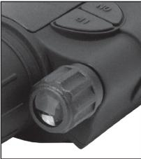
Infra-red illuminators, or IR illuminators, are common to night vision. The IR light greatly enhances the performance of the Viper X-1 while remaining almost totally invisible to the naked eye. The IR illuminator on the Viper X-1 is located underneath the front lens, next to the battery compartment.
