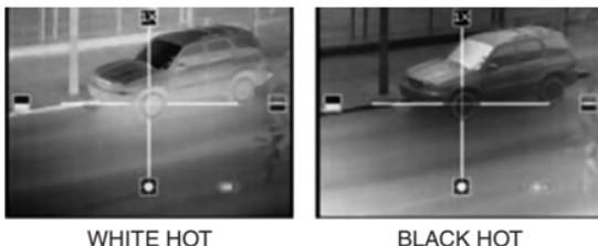
**FIGURE 3.7. DISPLAY POLARITY MODES**
