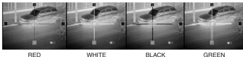
**FIGURE 3.11. RETICLE ADJUSTMENT**
