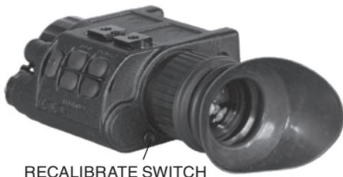
**Figure 3-4. Recalibrate Switch**
