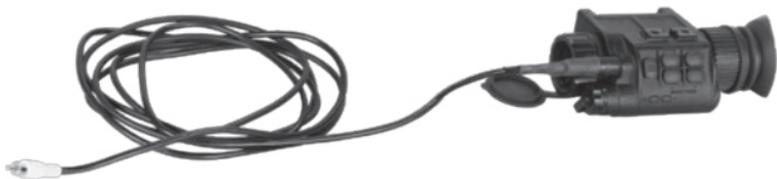
**Figure 2-2. Attaching Video Cable**
