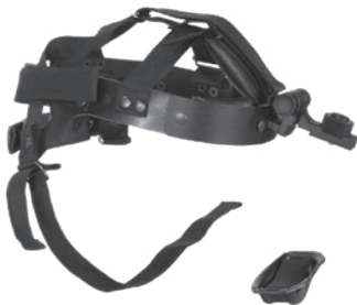
Figure 4-3. Removal and Installation of Chin Cup
