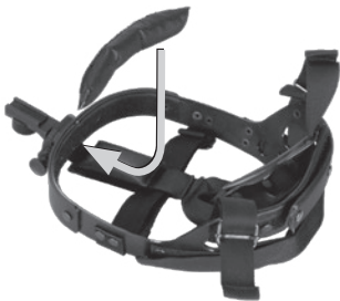
Figure 4-1. Removal and Installation of Browpad
