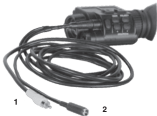
Figure 2-3. Attaching Video Cable
