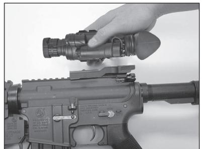
2. Align the monocular and the weapon mount. Slide the monocular rearwards until the alignment boss aligns with the alignment groove on the weapon mount. Push until the monocular locks into the weapon mount.
