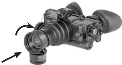
Figure 2-4. Installation of Compass
