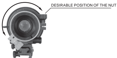
FIGURE 2-4. ESTIMATION OF THE ANGLE WHICH THE SCOPE MOUNTING SYSTEM SHOULD BE TURNED THROUGH
