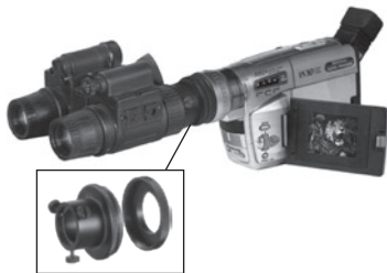
FIGURE 3-6. MOUNTING CAMCORDER TO THE ATN PS-15
