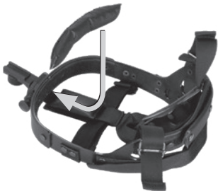
FIGURE 6-1. REMOVAL AND INSTALLATION OF BROWPAD
