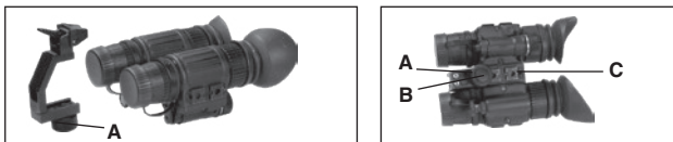
FIGURE 3-8. ATTACHING ADAPTER TO ATN PS-15
