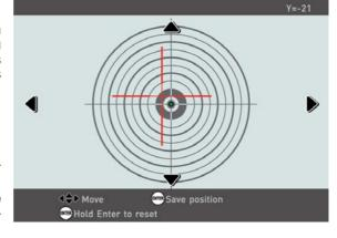
8. Using the keypad arrows, move your reticle to the point of impact and press "ENTER" to save the new reticle location. This will be your weapon's zero.
