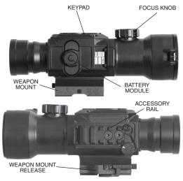
FIGURE 1.2. TICO MECHANICAL CONTROLS
