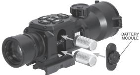
FIGURE 2.1. LOADING BATTERY MODULE
