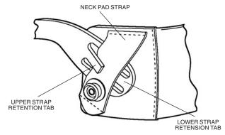
FIGURE 3.1. REINSTALLING THE NECK PAD
