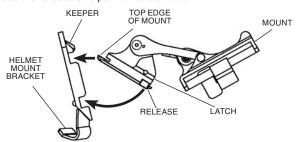
FIGURE 2.14. REASSEMBLY OF HELMET MOUNT
