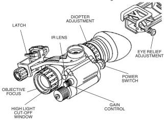
FIGURE 1.5. MECHANICAL FUNCTIONS FOR THE NVMPS
