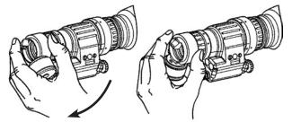
FIGURE 2.17. COMPASS INSTALLATION
