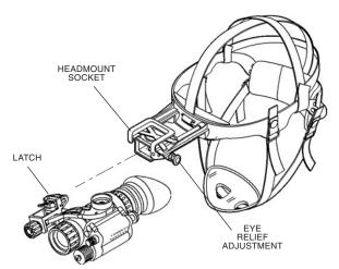
FIGURE 2.20. HEADMOUNT/HELMET MOUNT ADAPTER OPERATION
