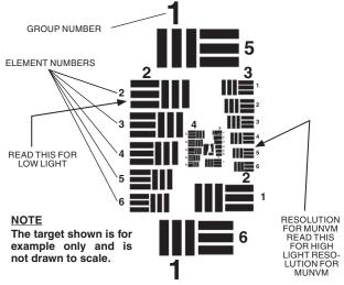
FIGURE 2.2. TS-4348/UV TEST SET PATTERN
