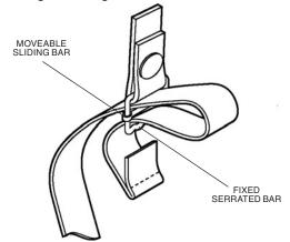
FIGURE 3.2. THREADING THE SLIDING BAR BUCKLES
