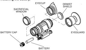
FIGURE 2.8. BATTERY, EYECUP AND EYEGUARD INSTALLATION
