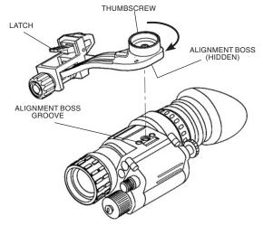
FIGURE 2.11. HEADMOUNT/HELMET MOUNT ADAPTER INSTALLATION
