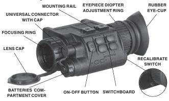
Figure 1-4. OTS Mechanical Controls
