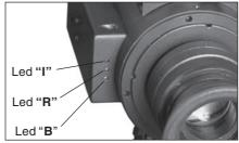
To adust the brightness of the reticle, or to turn It off all together, use the buttons located on the control box on the side of the unit Press and hold one of the + or adjustment buttons while the
