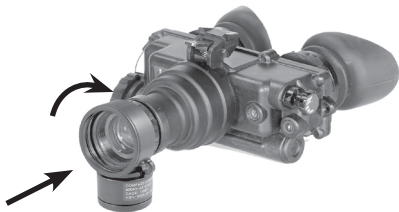
Figure 2-4. Installation of Compass
