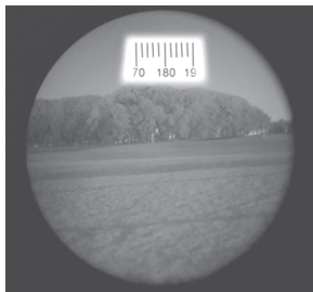
Figure 2-12. View Through Installed Compass
