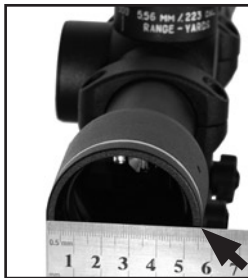
FIGURE B-1. OBJECTIVE TUBE DIAMETER MEASURING
