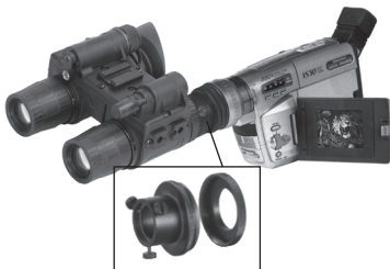
FIGURE 3-7. MOUNTING CAMCORDER TO THE ATN PS15
