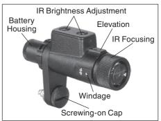
to focus on the scene observed in the viewfinder of your NVD. Use the included Allen wrench to rotate the adjusting screws until the IR beam is centered. Please remember the adjustments should be performed under night light conditions only.
