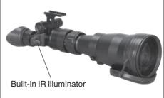
NOTE: The IR will automatically turn off when the unit's power is off.
